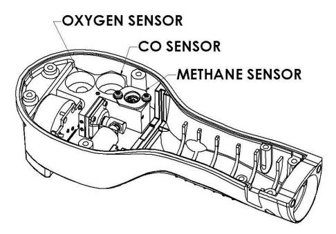
Figure 4. Gas-Explorer with top of case and main circuit board removed.
