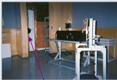
Projection through wave guide outside the magnet room
