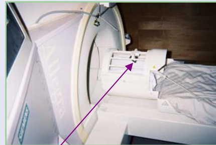
Stimulus mirror used to view display and track the eye
